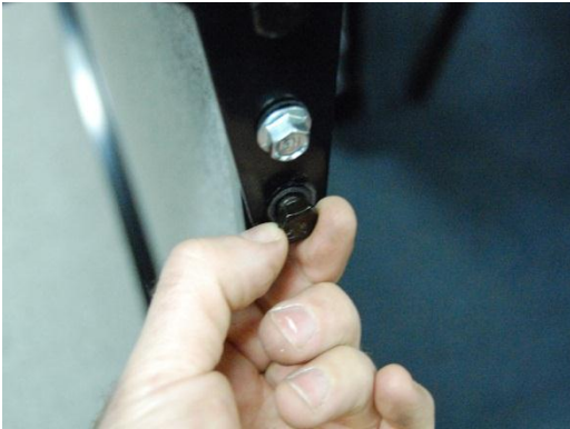
Step #12: Insert 9/16" bolt in top hole as shown, top and bottom.
