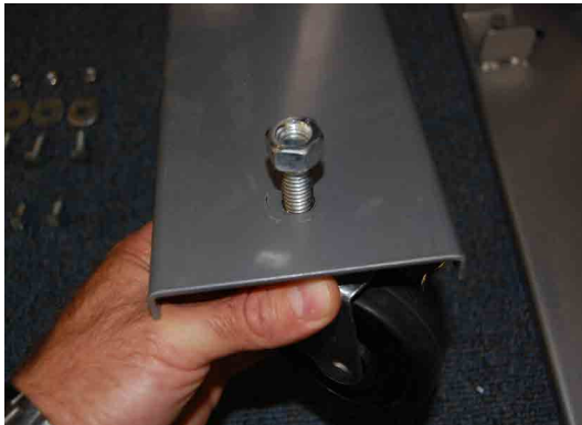
Step 1. Install caster to the end of the caster base closest to the unit to unit lock.
