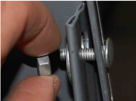
Step 7. From the back sided of the gate, attached the strut as shown. (handle end)
