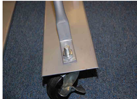
Step 2. Install second caster to the other end of the caster base and add the supports strut as shown. Repeat for all caster bases.
