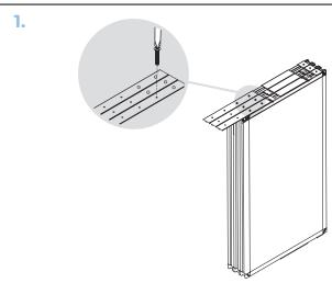
Remove the long bolt from the side of each of the top panels.\* Slide an end cap joint flat side up, extrusion facing down into each top panel. Align holes and insert two long bolts per panel.
