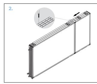
Remove a long bolt from each bottom panel. Slide top and bottom together with end cap joint, align holes and insert two long bolts per end cap joint on top panel.
