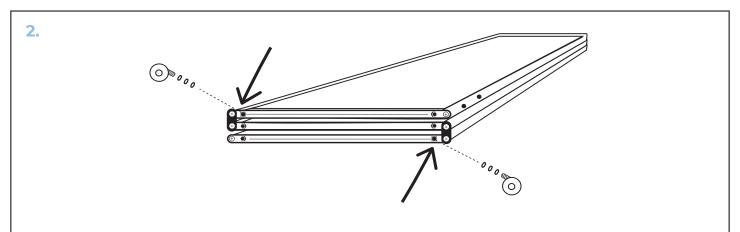
To attach wheel to panel, locate square nut in bottom track of outer panel and slide to outer edge. Add three washers to wheel threading and screw into square nut. Repeat for remaining wheels.
