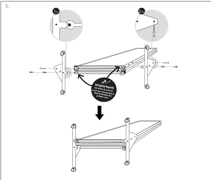
Remove two bolts from outside, bottom edge of each outer panel and one screw from the side of each outer panel. Then attach foot base with **bolts first**, screws second. Repeat for other side. Assembly complete.
