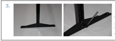
Position the foot assembly so the buttonhead of the two screws are on the outside of the Countertop Shield and slightly tighten each screw with the included allen wrench, do not fully tighten.
