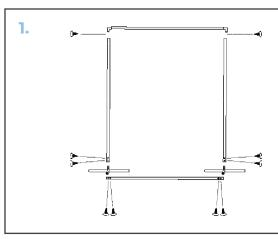
Layout poles in correct shape and screw in bolts to connect the polies together with the screws provided.
