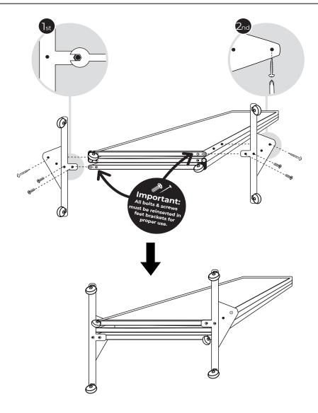
Remove two bolts from outside, bottom edge of each outer panel and one screw from the side of each outer panel. Then attach foot base with **bolts first**, screws second. Repeat for other side. Assembly complete.
