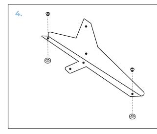
If not using wheels, insert button head screw down into foot end and secure with two washers and a nut. Repeat for other side of foot. Repeat for second foot.
